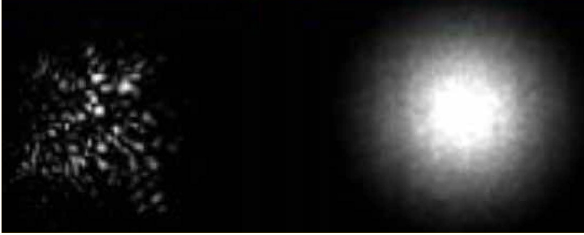
Figure 7.9: Left panel: short exposure speckle image. Right panel: long exposure showing the smoothed "seeing" disk of the observed point source.
